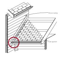
Kick-out flashing (seen in the red circle) diverts water away and the wall and into the gutter.
